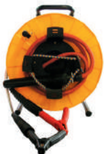
HSK 27B (for standard version): 25 m HV cable reel, crank handle, connection: 10 mm MC sockets incl. HV terminals and SE adaptors, approx. 17 kg
